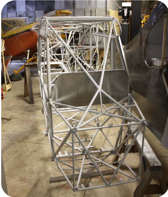
PA-18 FUSELAGE REBUILD READY FOR SHIPPING
